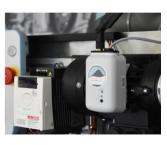
General machinery - Install in difficult to reach places, moving operations or dangerous spots and safely monitor from anywhere. Checkmate can use an accelerator to detect motion and easily by report abnormal movements
